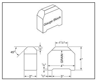
Figure 10. Guide block specifications.
